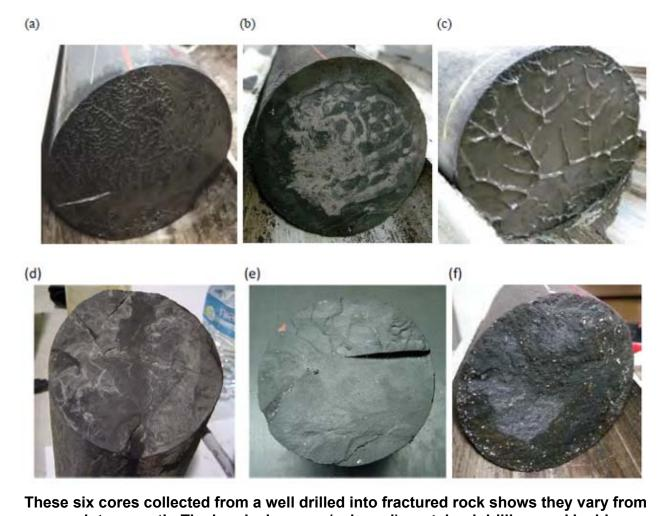
These six cores collected from a well drilled into fractured rock shows they vary from rough to smooth. The breaks in some (a, b, c, d) contained drilling mud inside.
